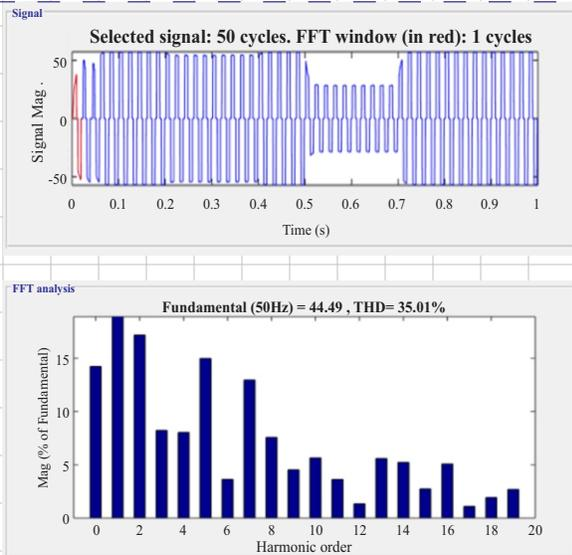
Fig. 7. Harmonic analysis source current without UPQC
