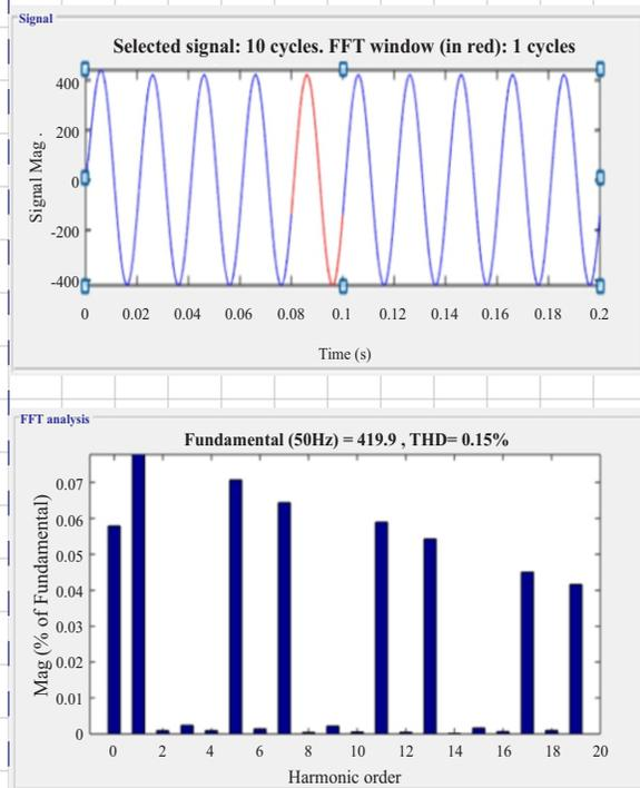
Fig. 10. Harmonic analysis source current with UPQC and FLC (zero angle)
