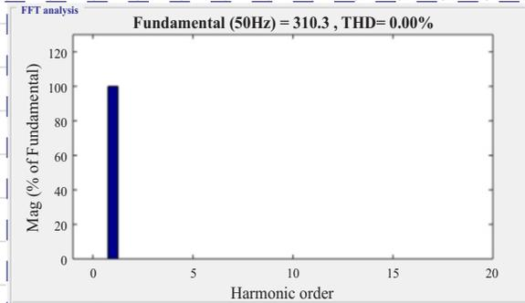
Fig. 9. Harmonic analysis source voltage with UPQC and FLC (zero angle)
