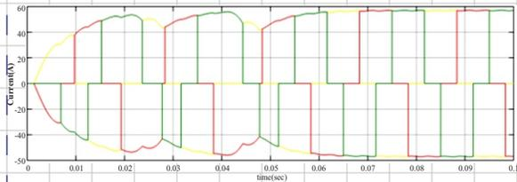
Fig. 14. Source current without UPQC (at zero angle)
