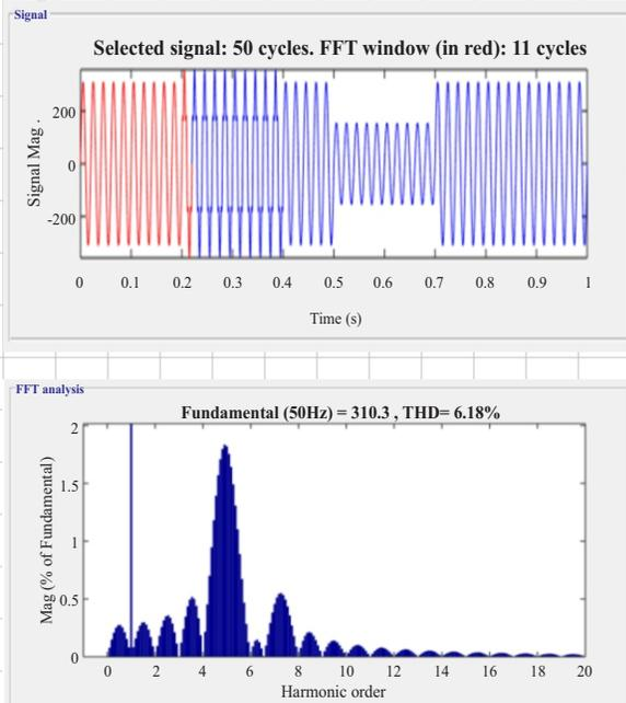
Fig. 8. Harmonic analysis source voltage without UPQC
