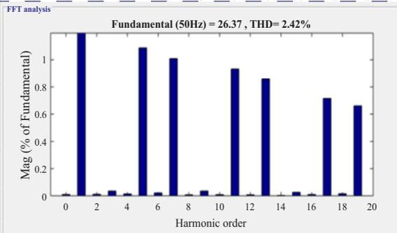
Fig. 11. Harmonic analysis load voltage with UPQC and FLC (zero angle)
