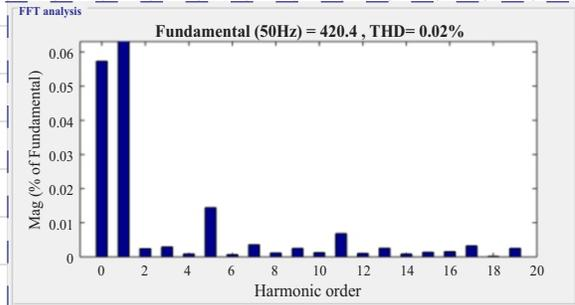
Fig. 13. Harmonic analysis Source current with UPQC and FLC (90 angle)
