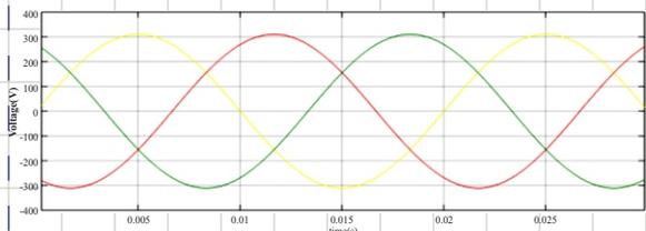
Fig. 16. Source voltage with UPQC (at zero angle)
