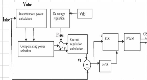
Fig. 4. Block diagram of shunt APF
