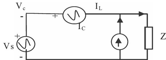
Fig. 2. UPQC: Equivalent circuit
