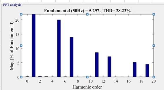
Fig. 12. Harmonic analysis load current with UPQC and FLC (zero angle)
