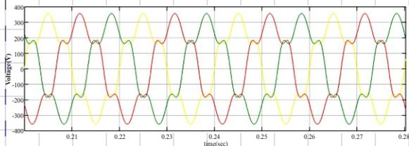
Fig. 15. Source voltage without UPQC (at zero angle)
